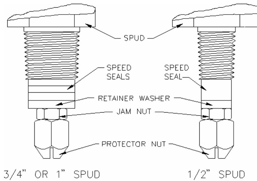
**Figure 4 - 6 Speed Seal Details**
