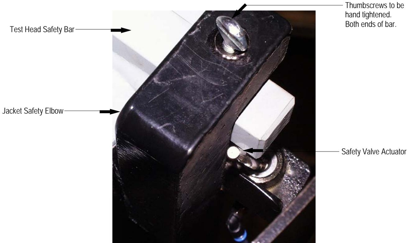
Figure 7-3 Interlock Actuator
