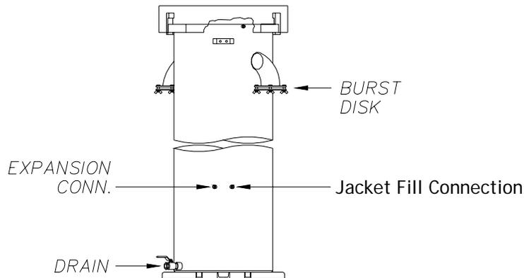
Figure 4 - 4 Hydraclose Test Jacket
