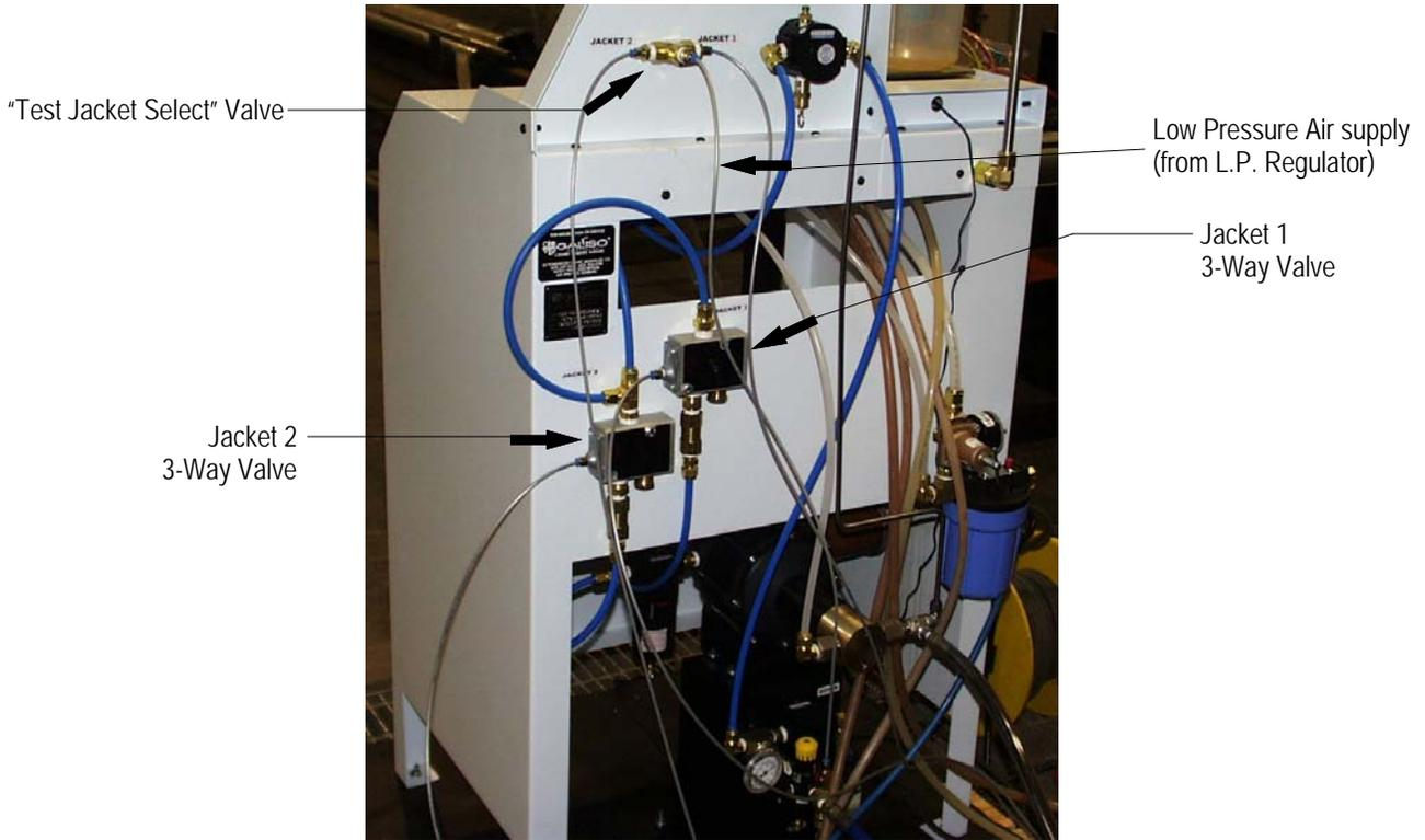
Figure 7-2 Interlock Parts-Rear of Console
