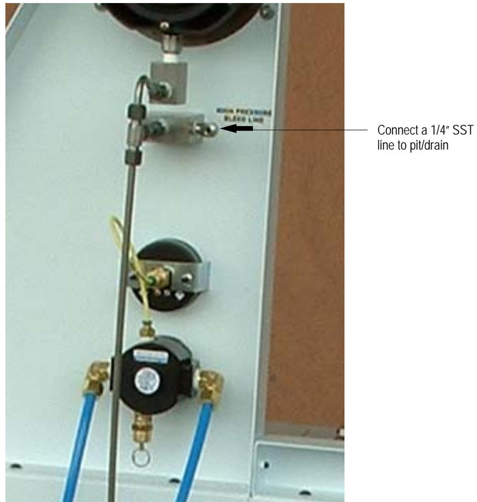
Figure 4-3b.1 Digital GTC Console Plumbing
