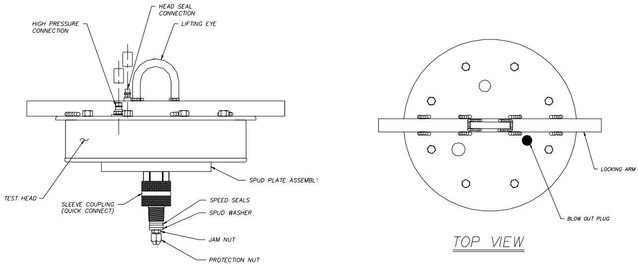
**Figure 4 - 5 Hydraclose Test Head**
