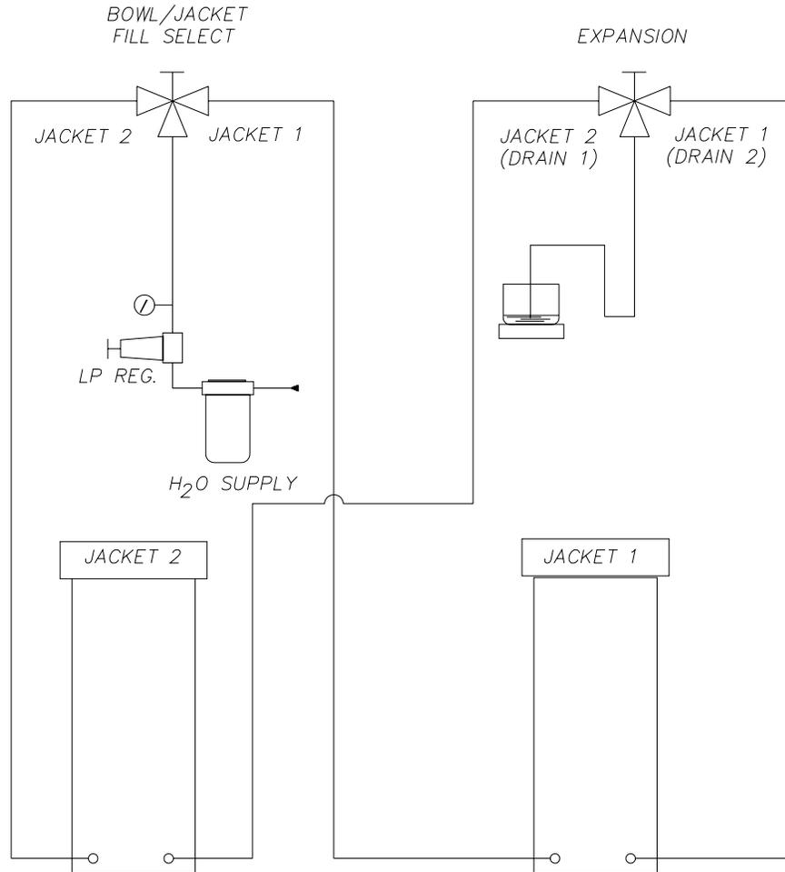
**Figure 4 - 7 Dual Jacket Schematic**
