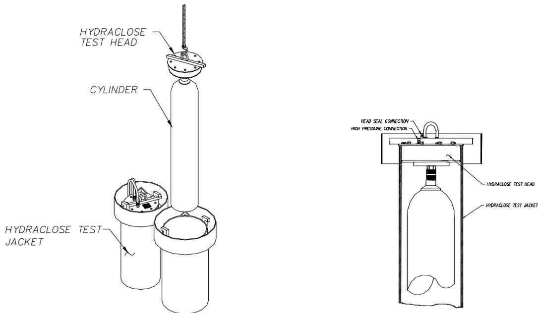
Figure 5 - 1 Cylinder/Test Head Installation
